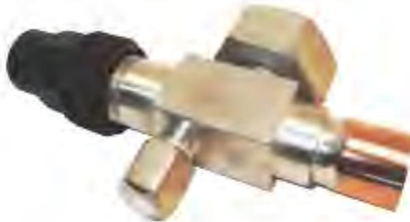
C&D Rotalock valves offer unsurpassed reliability, flow rate and corrosion resistance. Manufactured from carbon steel with a stainless-steel spindle and 100% copper connector they are first zinc plated and then tin plated.
